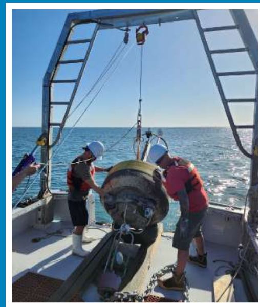
Images: CO-OPS' Currents Real-Time Buoy deployed near Jennettes Pier in Nags Head, North Carolina (left), CO-OPS field teams maneuver the buoy into the water (right).
