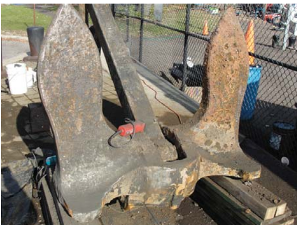
Cleaning the flukes, left one done, right one to be done next.
